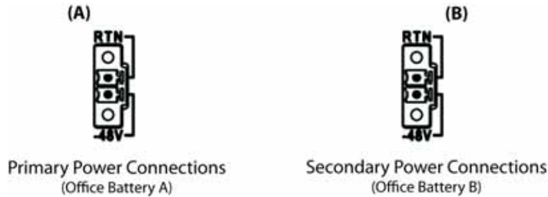
Figure 3-13. Power and Ground Connections on the TimeProvider 5000
